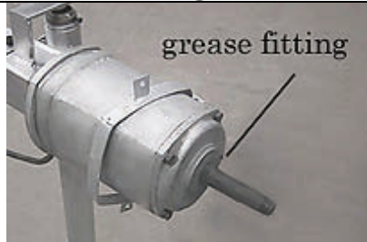
Models 800w-4.8kw This front bearing grease fitting is accessible with the body cover on. It is the same location on all models.
