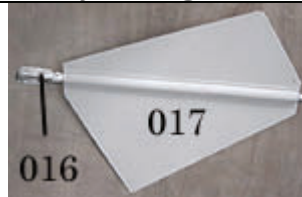
Models 800w-4.8kw Remove tail fin from the tail fin mount every 1-2 years and lightly apply grease by hand to the tail fin mount and bushings. DO NOT over grease this area.
