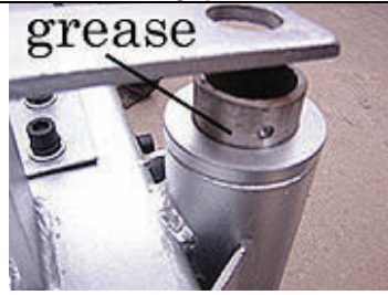
Models 800w-4.8kw Remove the Cyclone from the tower every 1-2 years and lightly apply grease by hand to the tower stub and bushings
